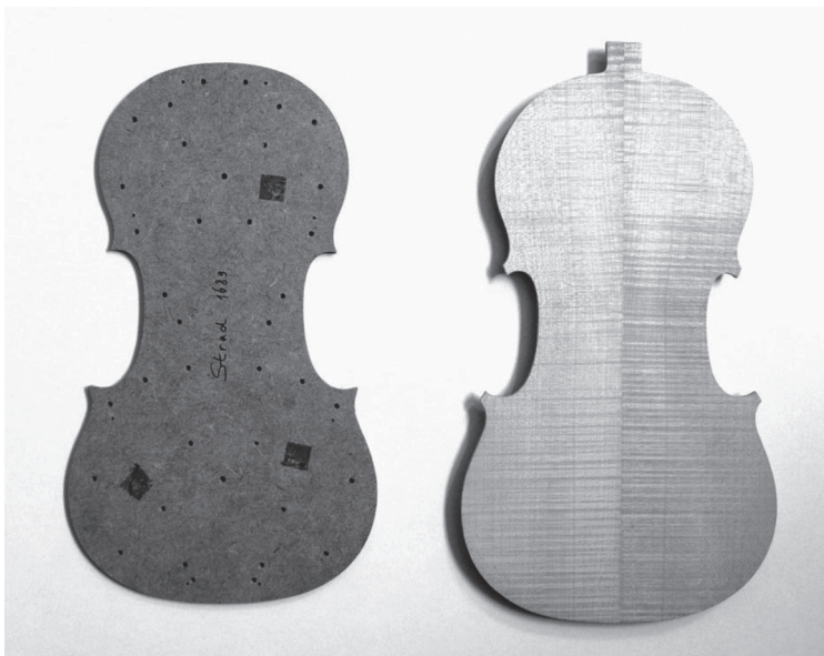
Figure 1 Template (left) and backplate (right) of base model after Antonio Stradivari 1689.
